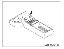
(1) When pressing the emergency switch downward the electric circuit is broken, all electrical function switch is off.
