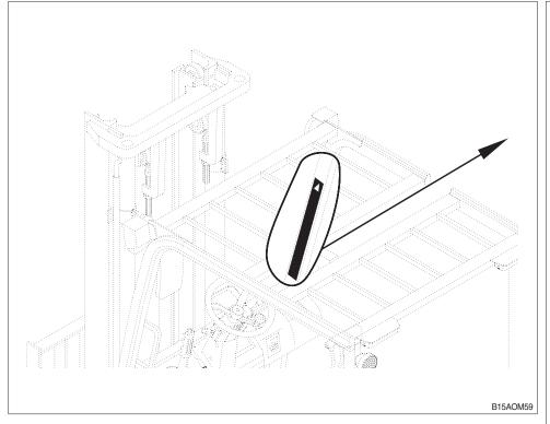
▲ Safety and warning decals are placed in conspicuous locations on the truck to remind you of essential procedures or to prevent you from making an error that could damage the truck or possibly cause personal injury. You should know, understand, and follow these instructions. Safety and warning decals should be replaced immediately if missing or defaced (Damaged or illegible). Refer to your parts manual for the location of all decals.
