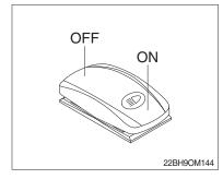
(1) This switch is used to operate head lamps. Press this switch to turn on head lamps.
