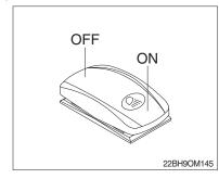
(1) This switch is used to operate work lamps. Press this switch to turn on work lamps.
