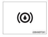
This LED lights when measured level of brake oil stored in reservoir tank is below the minimum acceptable mark.
